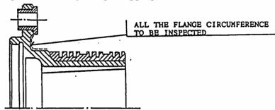
Remove the V 500A propeller so that the crack inspection may be performed. For propeller removing, see para. 2-2 "Disassembly of Propeller", 1991 issue of the "V 500A Propeller Operation Manual" p.15, or, as appropriate, Part "Disassembly of propeller Unit" in 1973 issue of the "V 500A Technical Description and Operation Instructions" p. 45.
